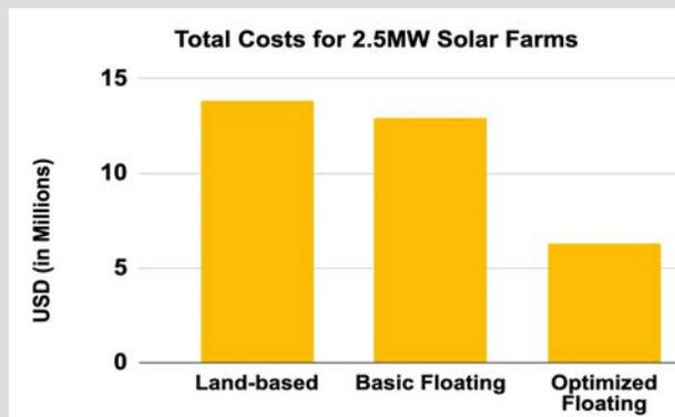
**Floating Solar provides significant economic advantages.** We performed a comparative economics analysis between land-based and floating solar. Total costs are for a 2.5MW plant and combine the costs of all solar panels & hardware with land or water acreage.
