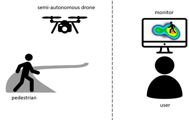
Visualization of pedestrian prediction and flight trajectory overlay on streaming video by using AR. Then, user can change confidence level of the prediction to avoid collision.
