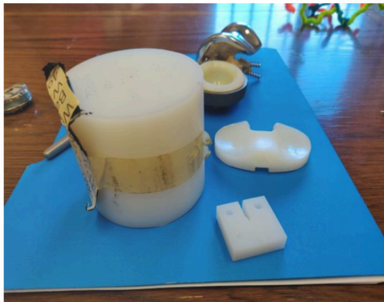
Figure 4. UHMWPE block (left) is carved into the tibial insert (right).
