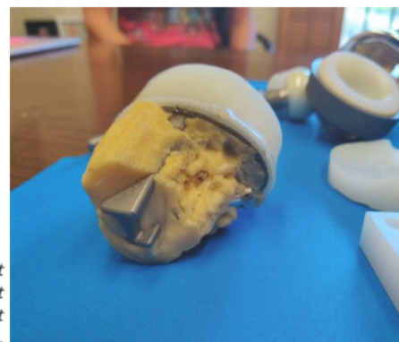
Figure 2. A retrieved tibial component that shows slight wear damage in vivo. Still intact are the bone fragments that were grafted out from the revision knee replacement surgery.
